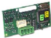
Fig. 4: Serial card for connection to a building management system or for master/slave control
